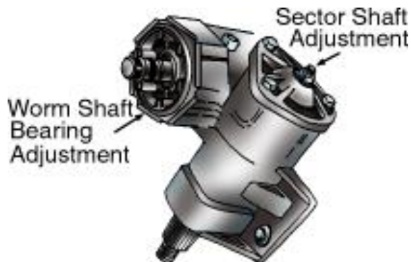
Gambar 174. Steering gear box.
