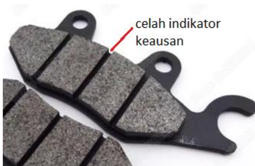
Gambar 2.15 Indikator keausan brake pad
