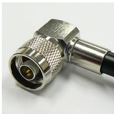
Right-Angle N-Type MALE Connector to suit RU400 or RG8 cable, crimp with solder pin
