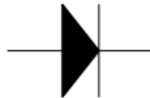
Gambar 6.23. Gambar Simbol Dioda
