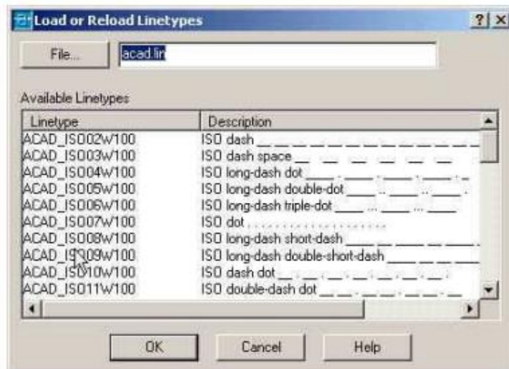
Gambar 6.19. Kotak dialog Load or Reload Linetypes
