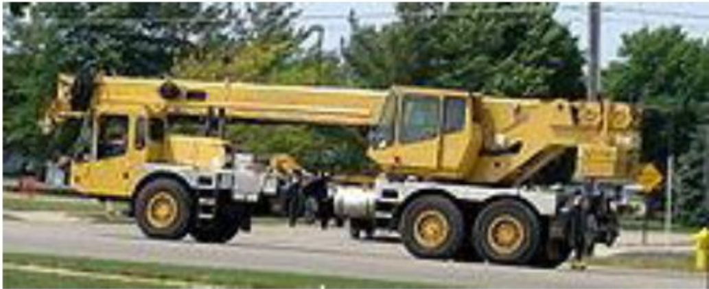
Gambar Truck mounted crane
