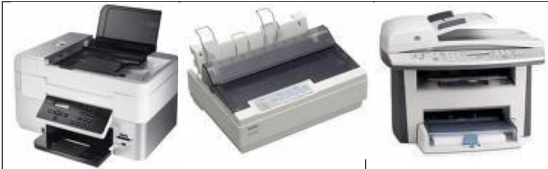
**Gambar 2. 8: model, printer tinta, dot matrix dan printer Laser**
