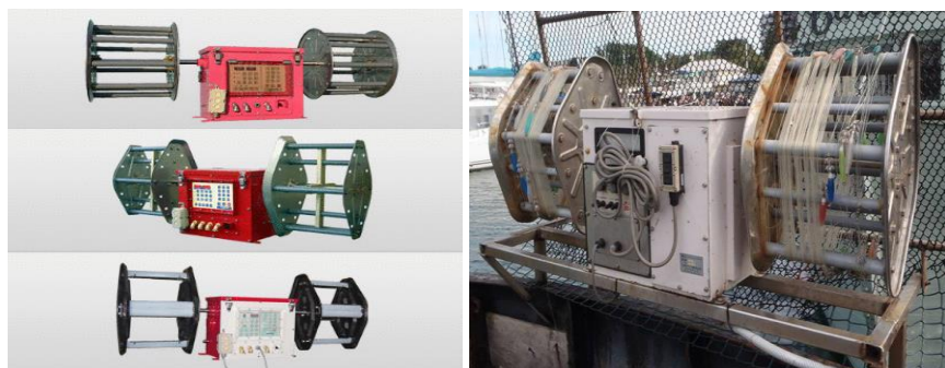
Gambar 166. Mesin pancing cumi otomatis (jigging automatic machine)
