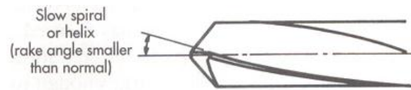
Gambar 2. 54 Mata borspiral panjang/ slow spiral
