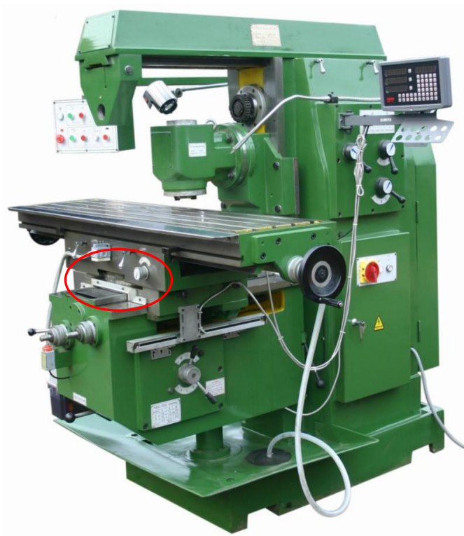
Gambar 3. 3 Mesin frais universal
