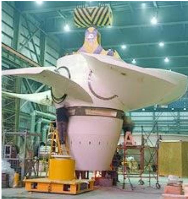
**Gambar 5. 5 Turbin Propeller jenis KAPLAN**
