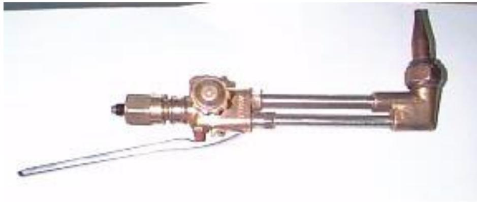
**Gambar 3. 14 Cutting blowpipe (pipa hembus pemotong)**
