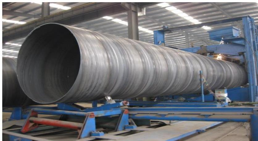
Gambar 3.8 Hasil Spiral Welded Pipe
