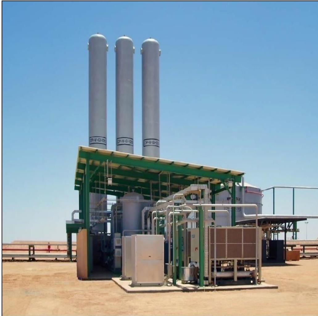
Gambar 7. Unit Nitrogen Plant (linde-engineering.com)
