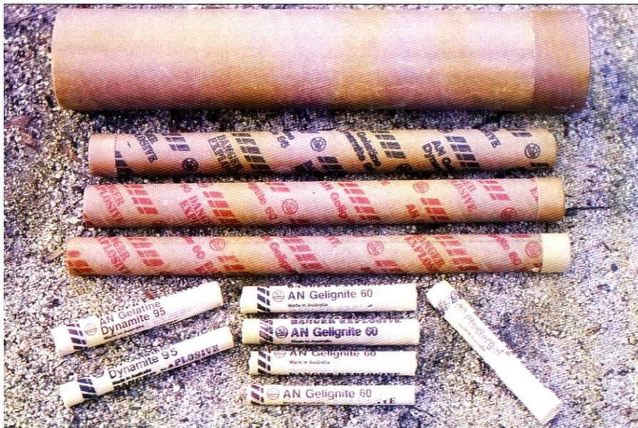
Gambar 6.13 Seri AN Gelignite buatan ICI Explosives (1988)
