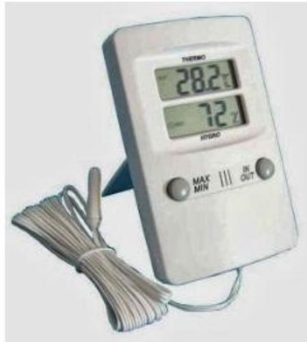
Gambar 20 Higrometer Digital
