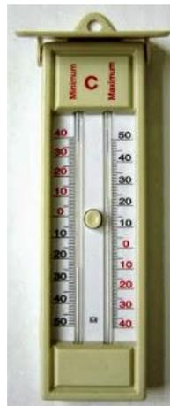
Gambar 10 Termometer Maksimum-Minimum
