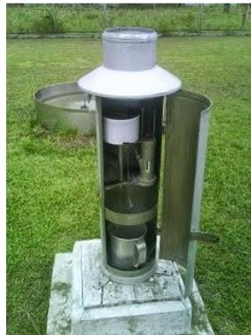
Gambar 24 Ombrometer tipe Hellman
