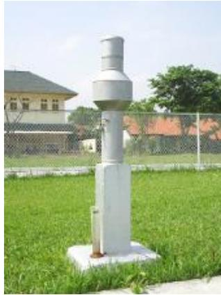
Gambar 22 Ombrometer tipe Observatorium
