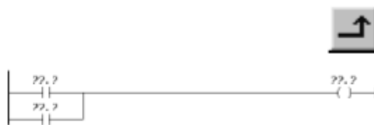
Gambar 19. Parallel ladder close branch
