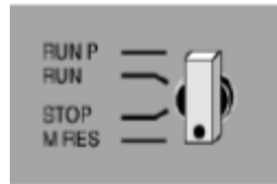
Gambar 36. Switch Mode PLC
