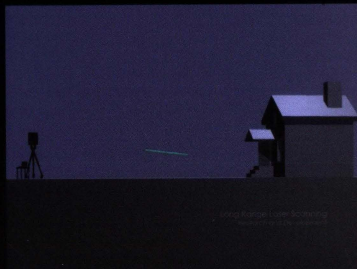
Gambar 2. Prinsip Kerja 3D Laser Scanning
