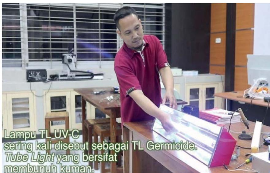
Gambar 3. Portable TL UV-C Germicide
