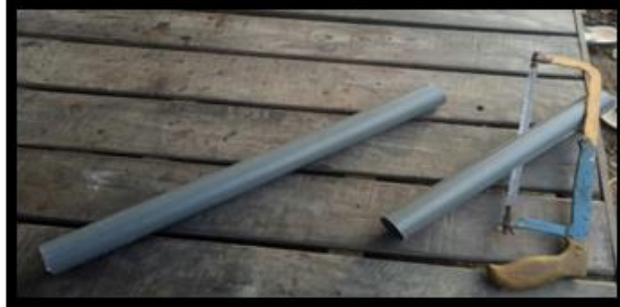
Gambar 2. Proses Memotong Pipa Paralon
