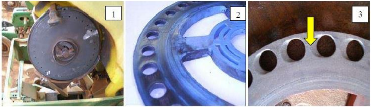
FIGURE 2. Metering mechanism of corn seeds: pneumatic with vertical perforated disc (1), horizontal perforated disc without (2) and with ramp ® (3) at the orifice exit.
