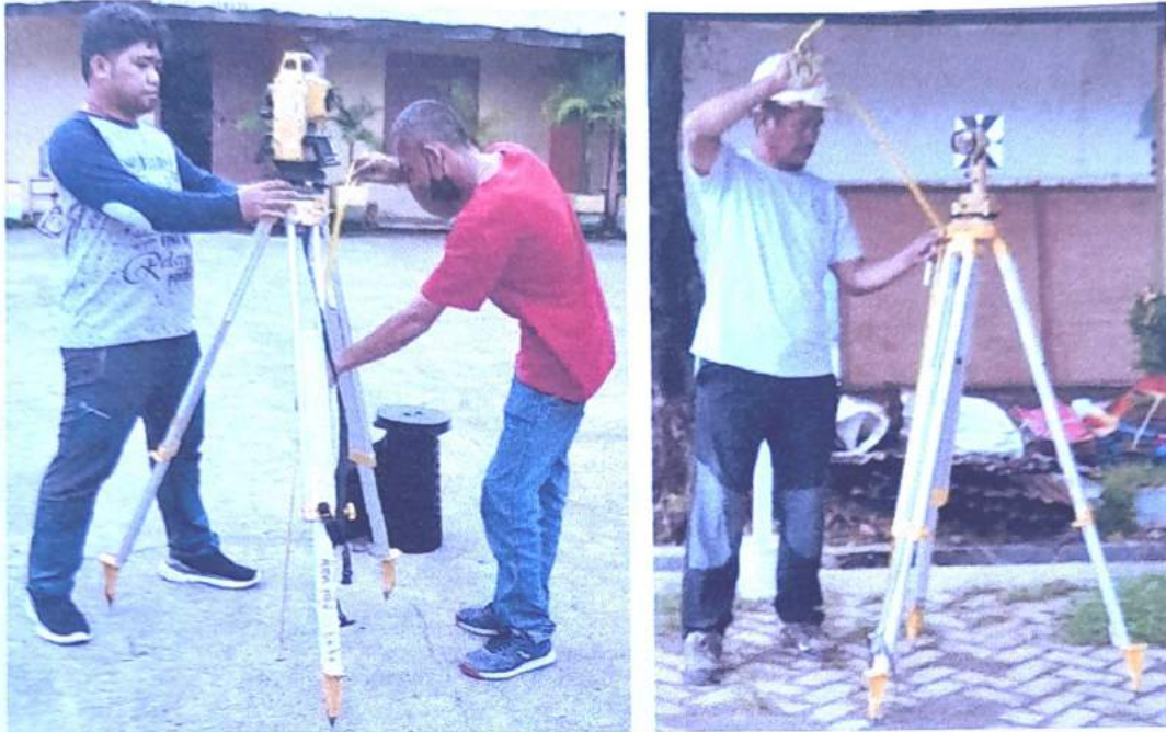
Setting awal alat total station sebelum operasional
