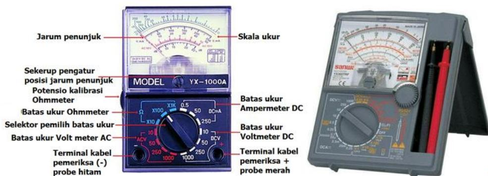
Gambar 33. Multimeter analog
