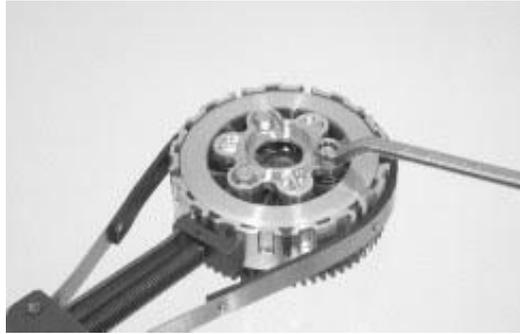
Gambar 2.15 Membongkar Unit Kopling.
