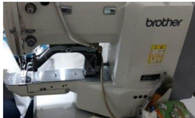
Gambar 6. 8: Mesin Jahit Trens (*Bartacking mechine*)
