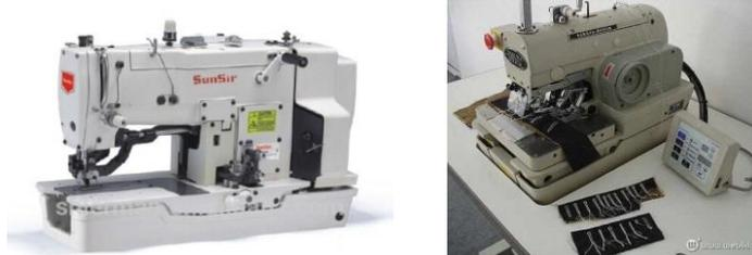
Gambar 6. 5: Mesin Lubang Kancing (*Button attaching*)
