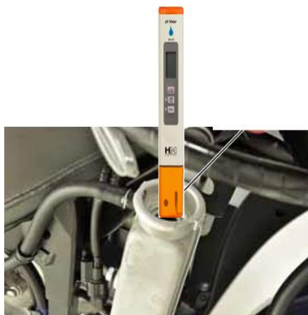
Gambar 2.29. Memeriksa pH air radiator
