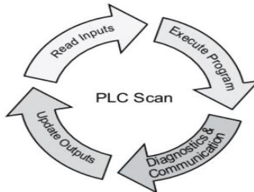
Gambar 77. Proses PLC scanning
