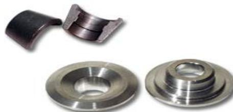
Gambar 2.9. Valve Keepers
