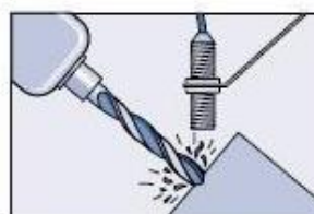
Application Detecting Broken Bit on Milling Machine Sensor 18 mm
