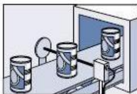
Application Counting Cans Sensor K50 Polarized Retroreflective
