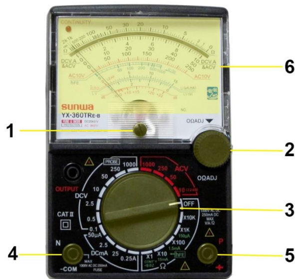
Gambar 2.4 Bagian-bagian multimeter analog
