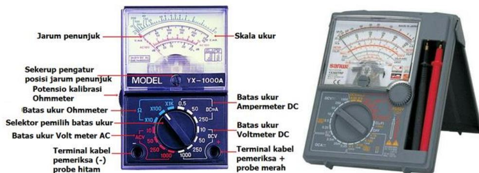
Gambar 45. Multimeter analog
