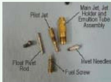
Gambar 13. Bagian-bagian main nozzle
