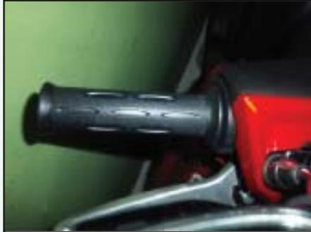
Gambar 50. Jarak main bebas gas tangan
