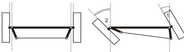
Gambar 24. Ackermann Steering Geometry
