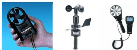
Gambar C.2 Anemometer Dan Data Logger
