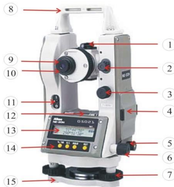
Gambar 10. Contoh theodolit digital
