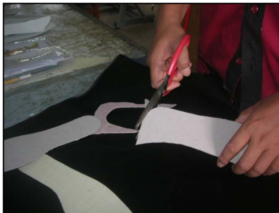
Gambar 5.48. Memotong in sole
