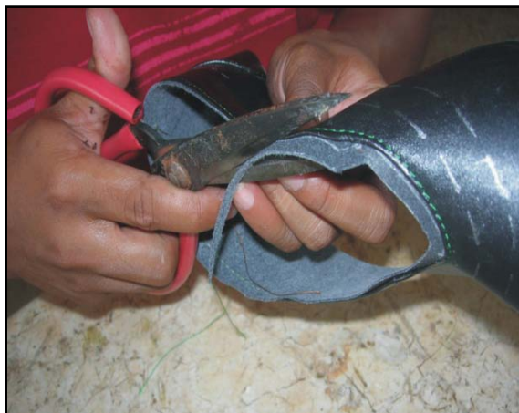
Gambar 3.54. Memotong kain lapis
